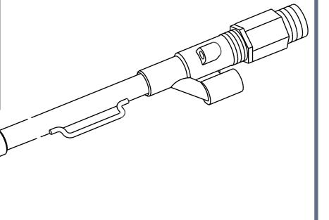
A mechanism in the head facilitates simultaneous suction cutting of yarn by pressing a button . It is possible to catch yarn in the traverse range .
